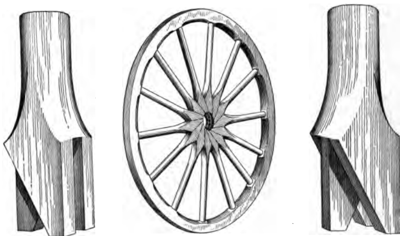
FIG 78.—Type of Wooden Artillery Wheel constructed with tongue-and-groove joints between the spoke wedges, ensuring greater strength and rigidity.
